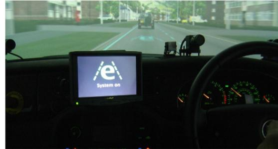
Figure 1. The in-vehicle interface
