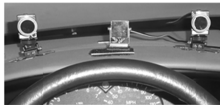
Figure 1b. Eye tracker on dashboard
