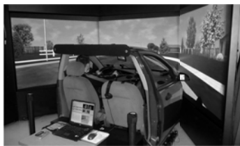
Figure 1a. Driving simulator
