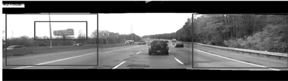
Figure 2. Panoramic video showing eye gaze direction (small circle near center) and ROIs for road ahead, left side of road, right side of road, and off-premise billboard (to the left)
