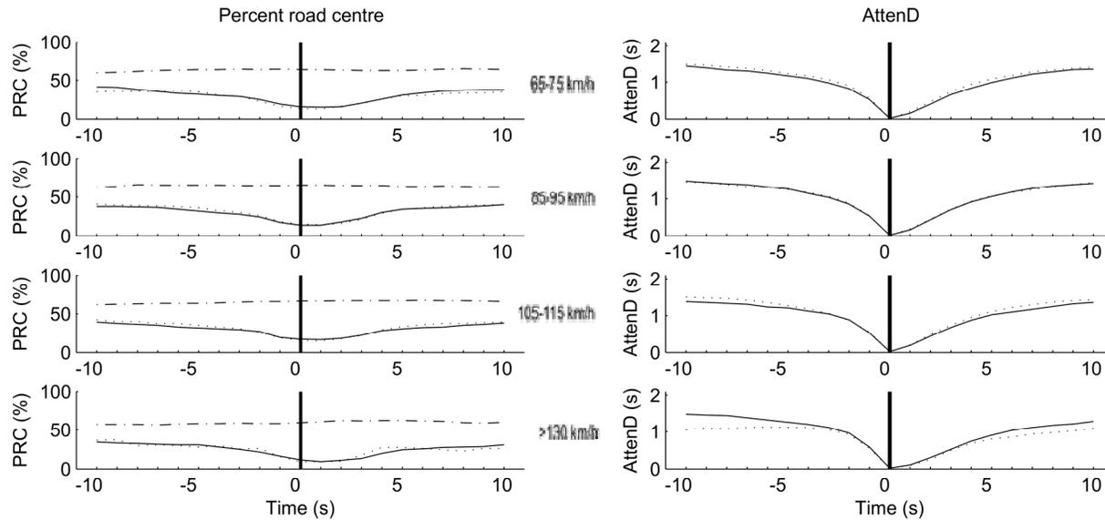
**Figure 1. PRC value (left) for cases of full attention (dash-dot line), and around warnings during baseline (solid line) and treatment (dashed line) for four speed intervals; average attention buffer (right) around warnings for baseline (solid line) and treatment (dashed line).**
